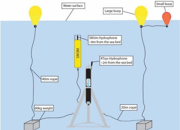
Indicative hydrophone schematic. However, the SM3M buoyant hydrophone will not be utilised in this instance.
