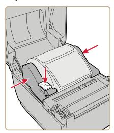
**4** If you are using notched or black mark stock, slide the label stop sensor so the notches or marks pass over the sensor.
