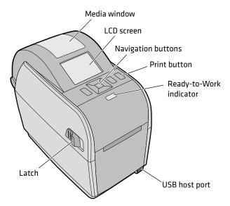
PC23d Front Panel (LCD Model)
