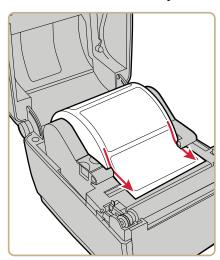
For a PC43t, thread the media through the media guides and past the front of the printer. To adjust the width of the media guides, slide the guides as needed to fit your media.
