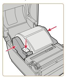
**4** If you are using notched or black mark stock, slide the gap sensor so the notches or marks pass over the sensor.
