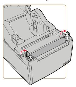
**5** Pull the latches up to remove the platen roller from the printer.
