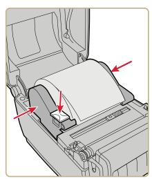
**4** For the PC43d, thread the media under the tip guides on the media holders.
