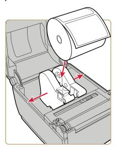
**4** Make sure the holders are snug against the sides of the media roll, and then press the locking tab down to lock the media holders in place.
