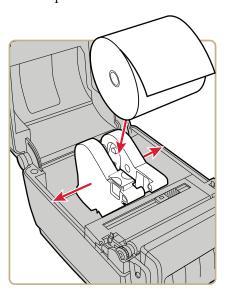
**c** Make sure the media holders are snug against the sides of the media roll, and press the tab down to lock the holders in place.
