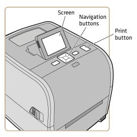
PC43t Printer with LCD Interface
