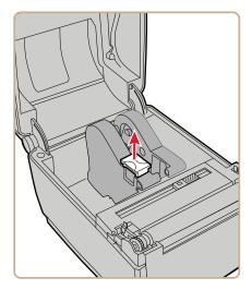
**3** Slide the media holders to adjust the distance between them, and place the media roll between the holders.
