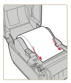
For the PC43t, thread the media through the media guides. To adjust the width of the media guides, slide the guides as needed to fit your media.
