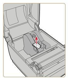
**b** Slide the media holders to adjust the distance between them, and place the media roll between the holders.
