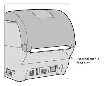
**3** Thread the media through the media holders or media guides as you would for media installed inside the printer.
