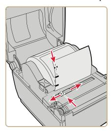
**5** For the PC23d and PC43d, thread the media under the tip guides on the media holders and past the front of the printer.
