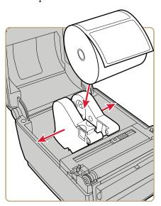
**c** Make sure the holders are snug against the sides of the media roll, and press the tab down to lock the holders in place.
