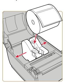
**c** Make sure the media holders are snug against the sides of the media roll, and press the tab down to lock the media holders in place.
