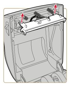
**5** Disconnect the cable from the printhead and remove the printhead from the printer.
