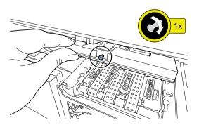
7. Connect Relay Harness connector to the printer.
